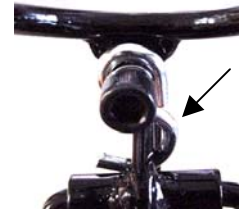
Fig. 2 Hook-Set Feature Locked Out For Use As Stationary Rod Holder
